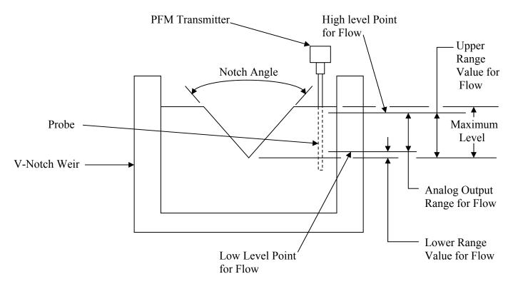
Determine the Maximum Level. This is the highest point that can possibly be measured. This is usually, but not always, the same as the height of the throat. Fill in the value below.
